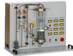
**AIM:** to demonstrate the different condensation processes using two tubular shaped water-cooled condensers made of different materials. Drop-wise condensation can be demonstrated by means of the condenser with a polished gold-plated surface. Film condensation forms on the matt copper surface of the second condenser, thus making it possible to examine film condensation.
