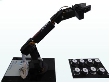
The PT-CIM 2C trainer can be expanded by using the PTR 4D robotic arm module. It provides to the students training in integrating a Robotic operation in the PT-CIM 2C process. The robotic arm operates as a palletizer or feeder to a follow-up process allowing the students to integrate a linear transfer system with a 4 degrees of freedom robotic operation. For more information on this module, please see the PTR 4D section
