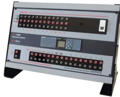
The PT 1208 Universal trainer is a programmable Logic Controller Trainer that combines high performance and easy of use operation for training students in PLC operation and programming.
